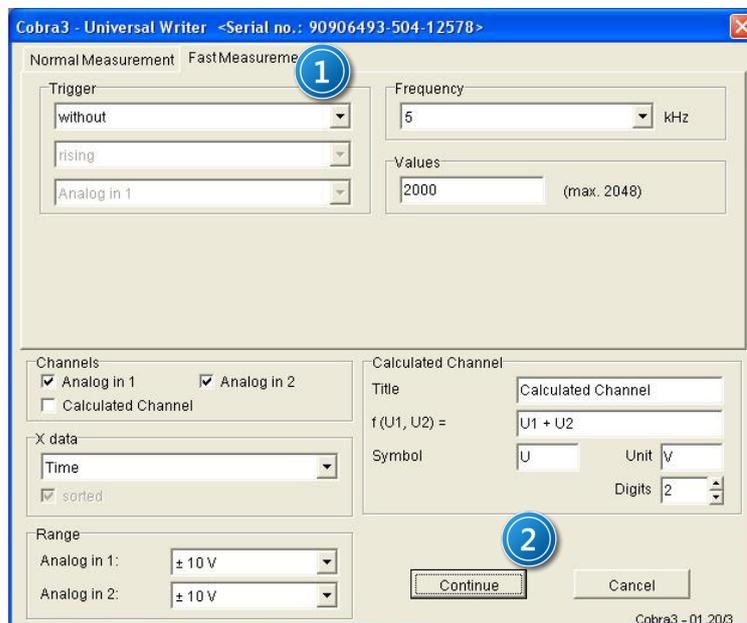
Picture 9. Cobra 3 window: - Universal Writer: 1 - Fast Measurement tab; 2 – confirm changes.
