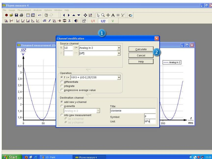
Picture 13. Window for voltage-volume conversion: 1 – selected channel U2; 2 – confirm changes button.
