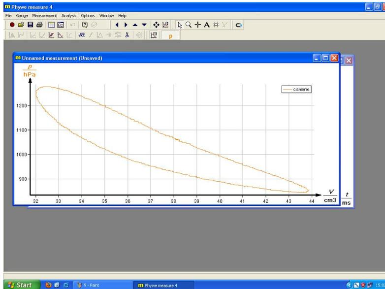
Picture 17. Correctly obtained pV diagram.
