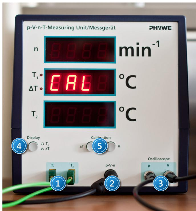
Picture 3. p-V-n-T meter: 1 – thermocouple inputs  $T_1$ ,  $T_2$ ; 2 - p-V-n meter cable input; 3 – oscilloscope output p and V; 4 – temperature display mode selector switch; 5 – temperature and volume calibration buttons.
