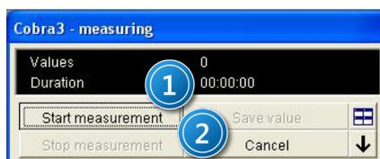
Picture 10. Cobra 3 – measuring window: 1 – start measurements button; 2 – stop measurements button.
