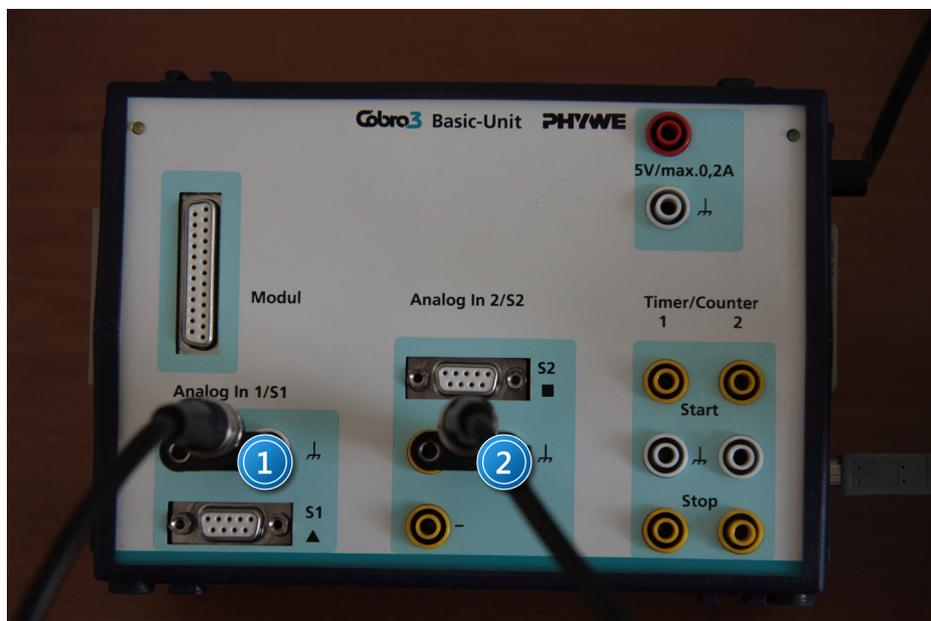
Picture 6. Cobra 3 measuring unit: 1 – input Analog In 1; 2 - input Analog In 2.
