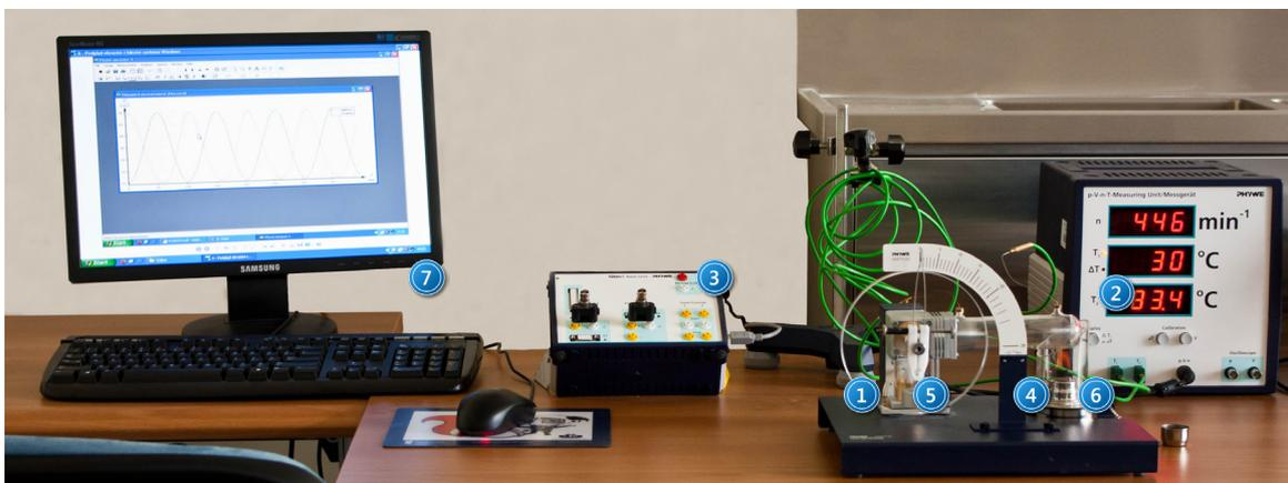
Picture 1. Measuring system with Stirling engine and Cobra 3 module: 1 – Stirling engine model; 2 –p-V-n-T meter; 3 – Cobra 3 measurement module ; 4 – torque measuring scale; 5 - torque-meter; 6 - burner with chimney; 7 - computer.
