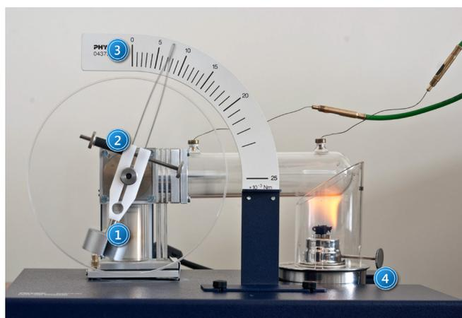
Picture 1. Operating Stirling engine: 1 – torque-meter; 2 – adjustment screw; 3 – measuring scale; 4 – burner with chimney.
