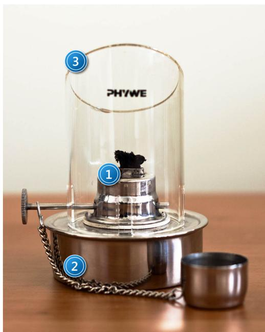
Picture 2. View of the burner: 1 – screw-cap; 2 - container; 3 - chimney.
