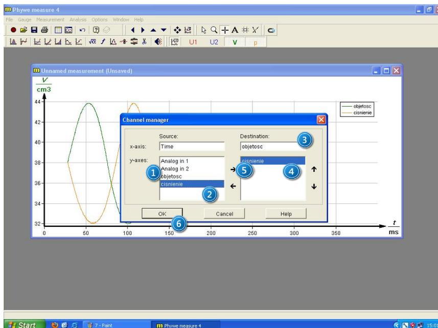
Picture 15. Graph transformation in XY mode: 1 – volume channel; 2 - pressure channel; 3 – assign channel to X axis; 4 – assign channel to Y axis; 5 – select channel; 6 – save changes.
