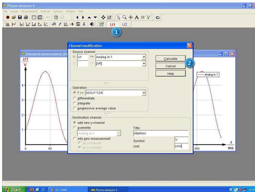
Picture 12. Window for voltage-volume conversion: 1 – selected channel  $U_1$ ; 2 – confirm changes button.
