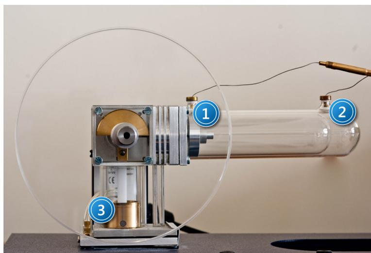
Picture 4. Model Stirling engine with vertical piston in the lower position: 1 – thermocouple  $T_1$ ; 2 – thermocouple  $T_2$ ; 3 – vertical piston in the down position.
