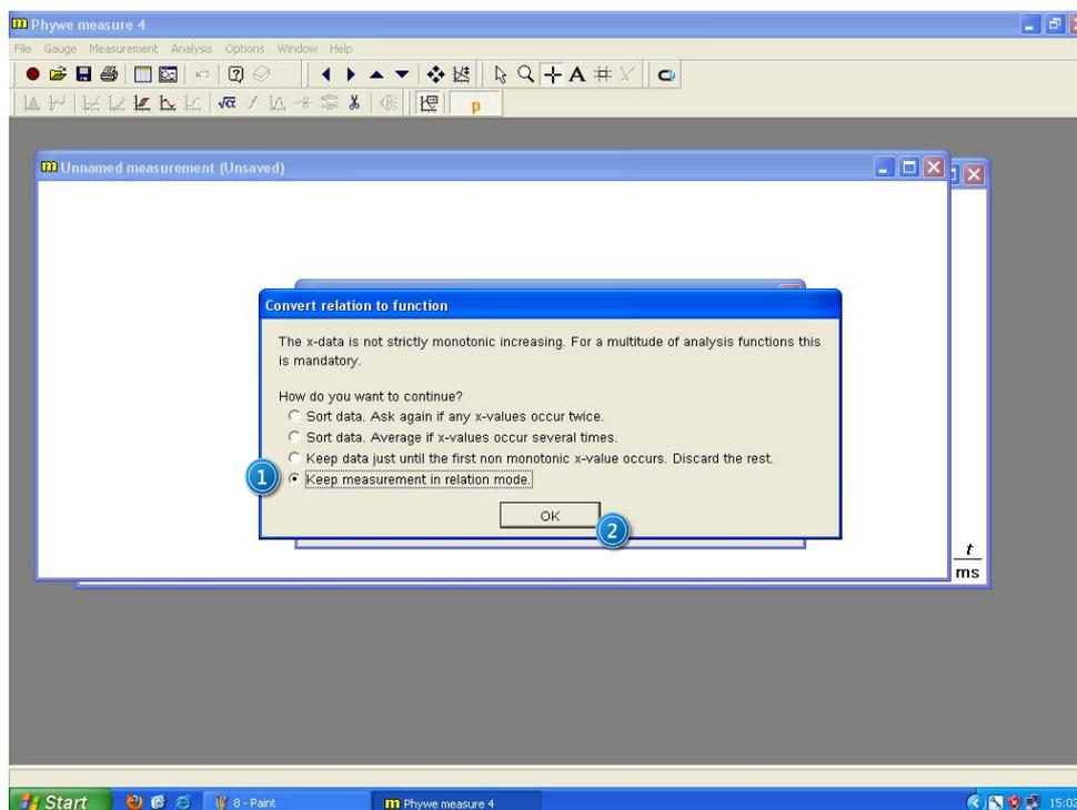
Picture 16. Setting the relationship between the channels  $U_1$  and  $U_2$ : 1 - Keep measurement in relation mode option; 2 – confirm changes.
