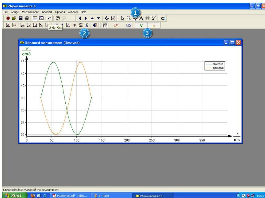
Picture 14. A single engine cycle: 1 – Mark tool; 2 – Cut tool; 3 – selected channels V and p.
