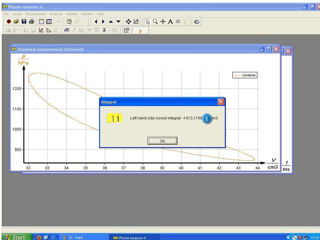
Picture 18. The area under the pV diagram: 1 – field value.
